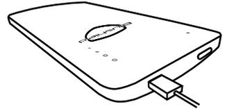
Push the ON/OFF button once to see the LED charging lights **D** light up. One LED will be flashing. This indicates the charging level. Once fully charged the LEDs **D** will no longer flash and four LEDs will be lit. This indicates that the portable is fully charged.
