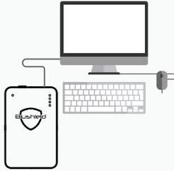
Firstly charge the Blushield Portable using the USB cable. Insert the small end of the USB cable into the slot **C** and the larger end into a USB socket on your computer or any phone charger sporting a USB socket.
